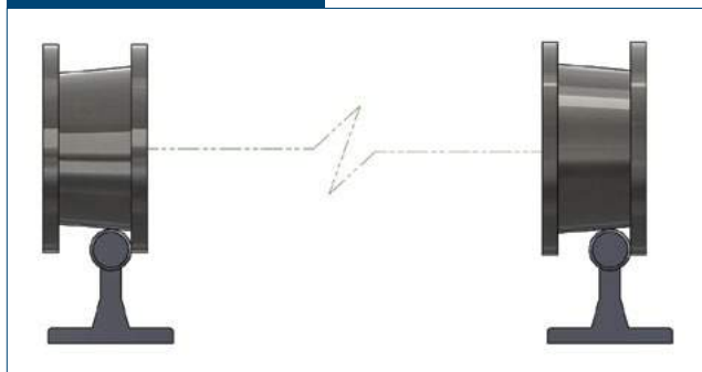
With the wheels traveling “out of the page,” the left wheel travels farther with each revolution; therefore, the wheels steer to the right and the idlers will follow. The crane will center on the rails as the active diameters equalize.
